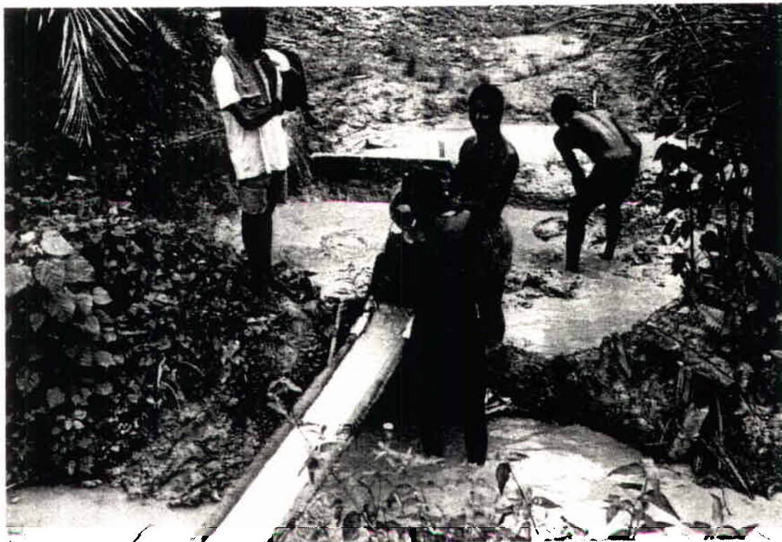
Water control and preconcentrating system of an alluvial gold sluicing operation in Ghana
