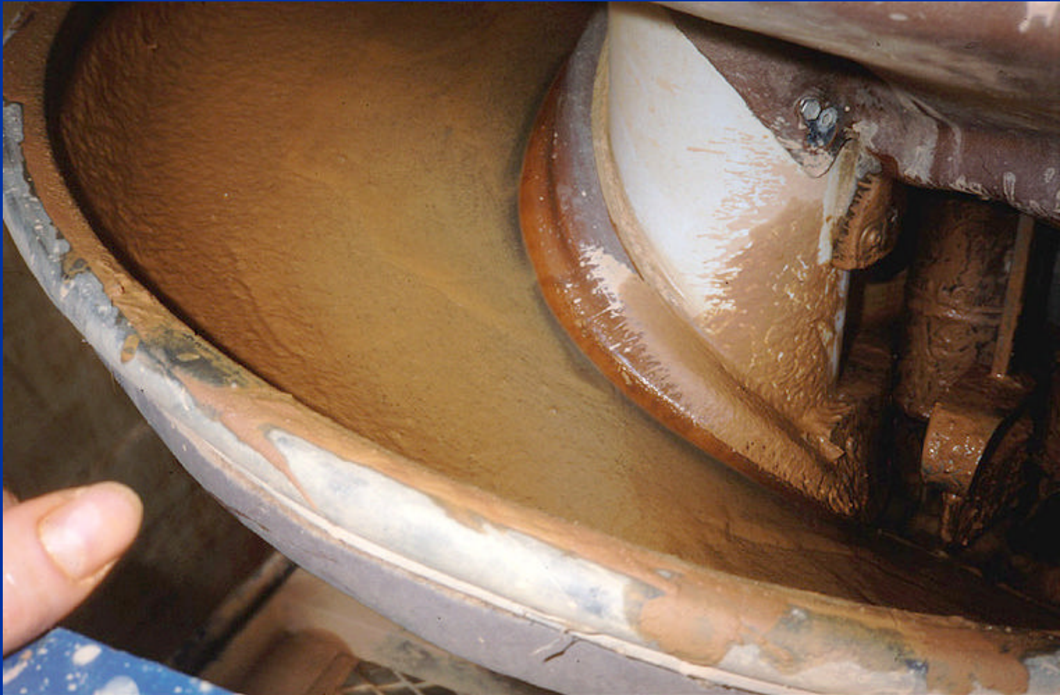
Spiral splitter setting (oxidised primary gold ore)
