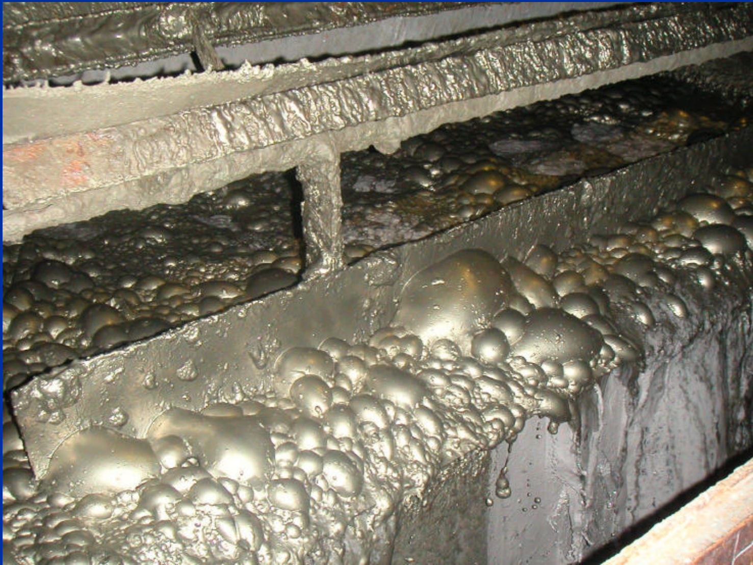
Flotation cell floating gold bearing sulfide concentrate
