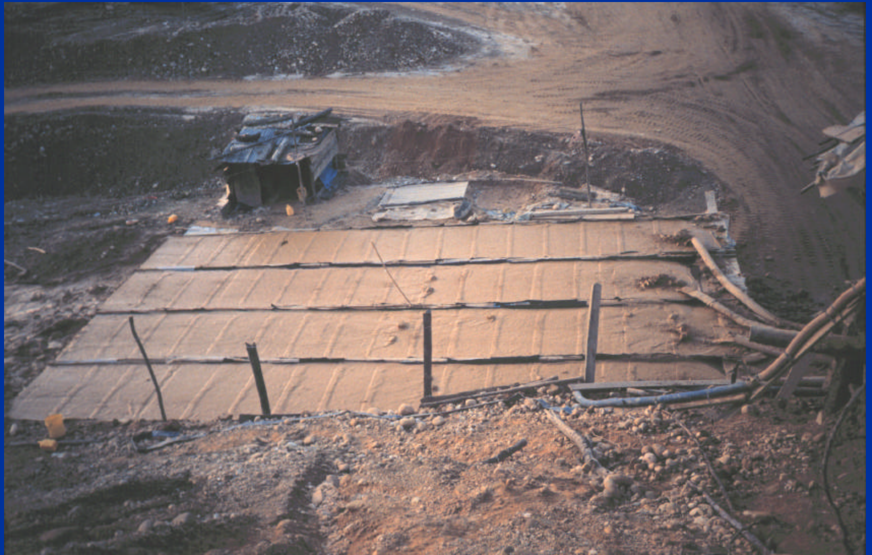
„carpet-only“ sluicebox for fine alluvial gold
