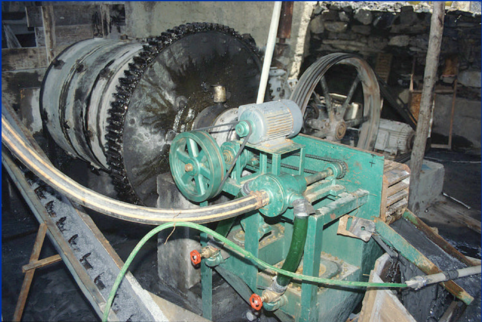
Jig (Type Denver Mineral Jig) in closed milling circuit (gold)
