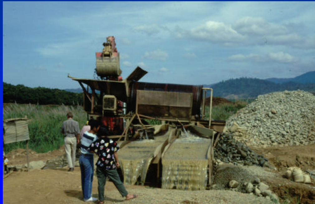
Jig (Ruby mining), combined with scrubber/trommel screen
