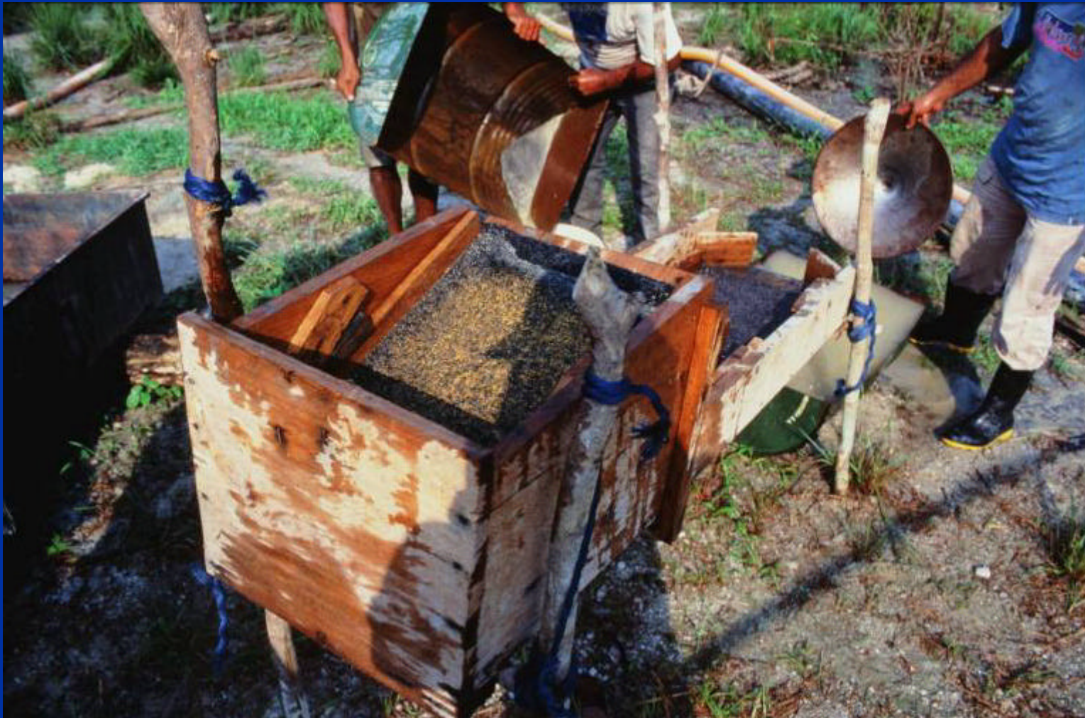
Sluicebox for cleaning alluvial pre-concentrate
