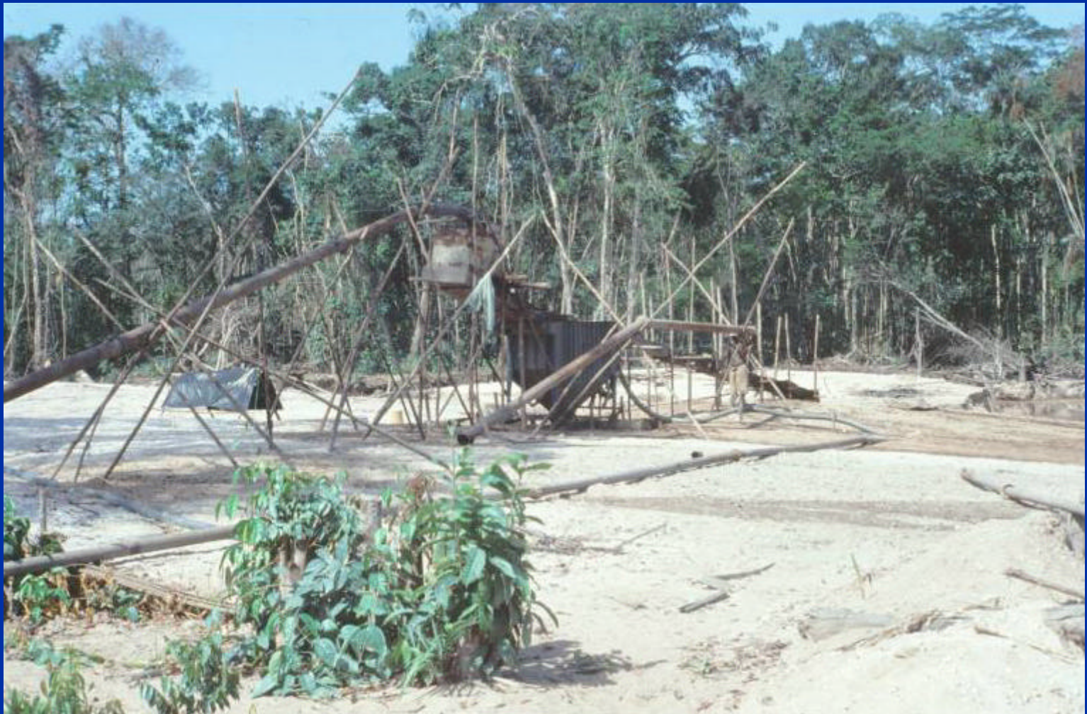
Jig (Type Panamerican) in alluvial diamonds processing
