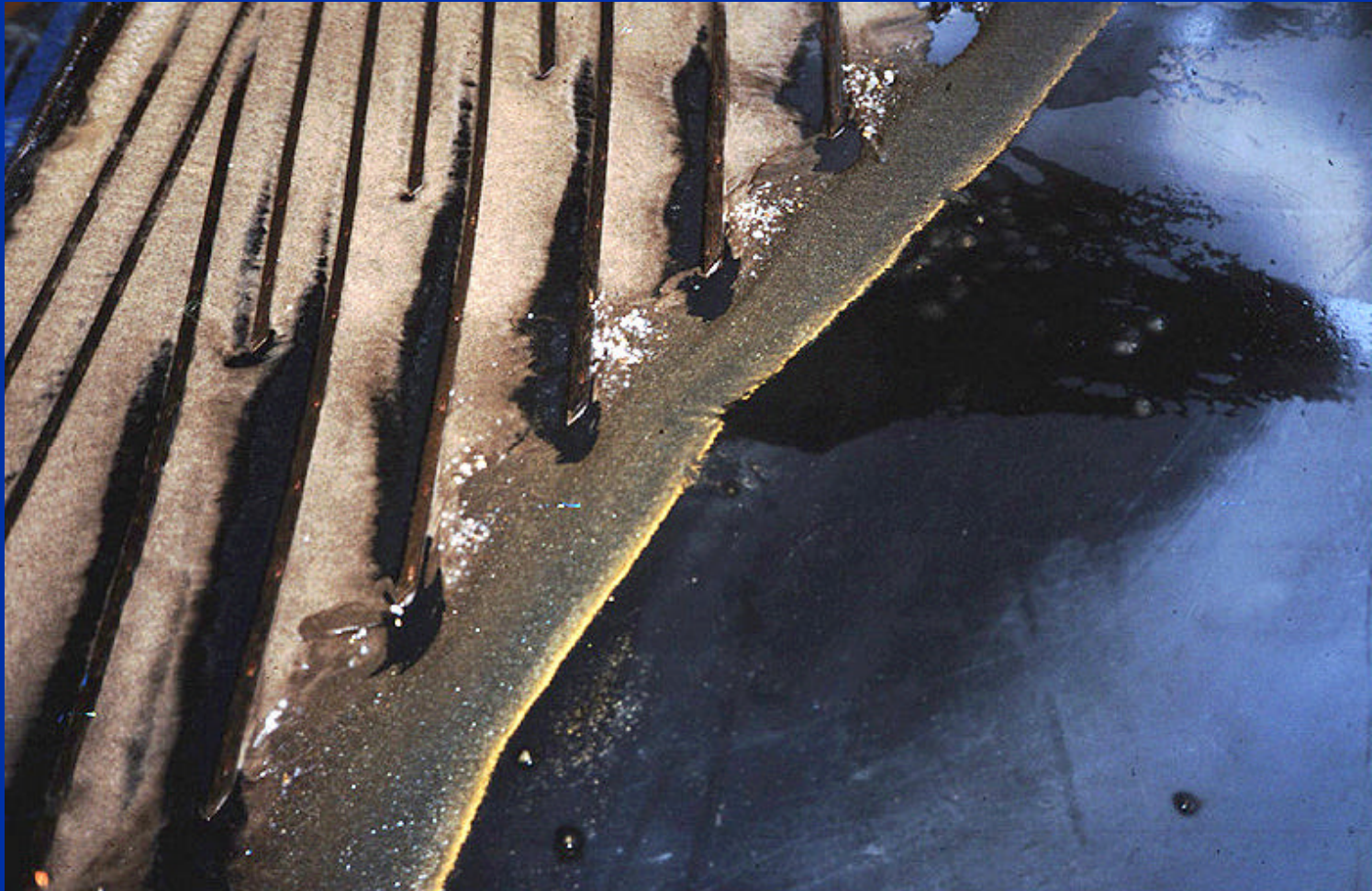
Gold, heavy minerals and quartz on shaking table (operation stopped)
