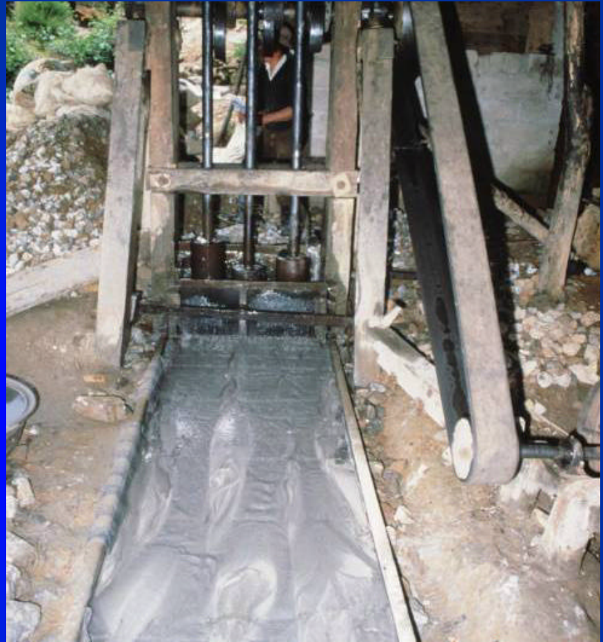
Stamp mill (iron, driven by electrical motor)
