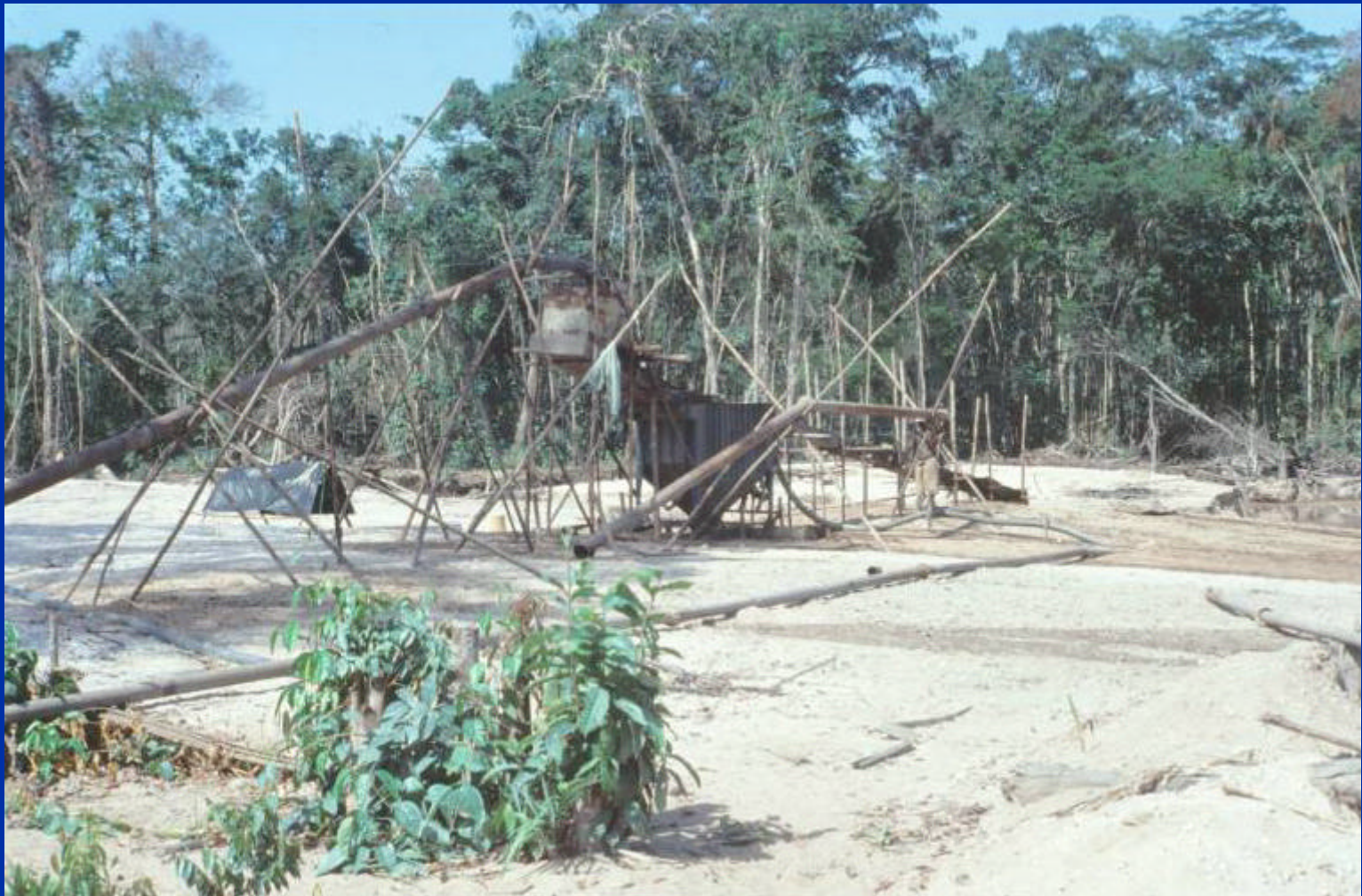
Jig (Type Panamerican) in alluvial diamonds processing
