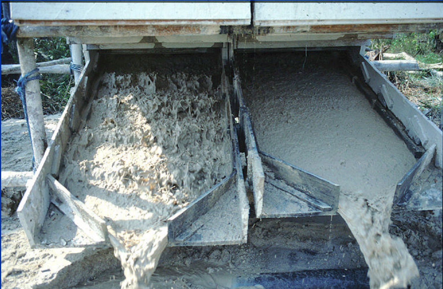
Test Sluice Box (left: turbulent, right: laminar)
