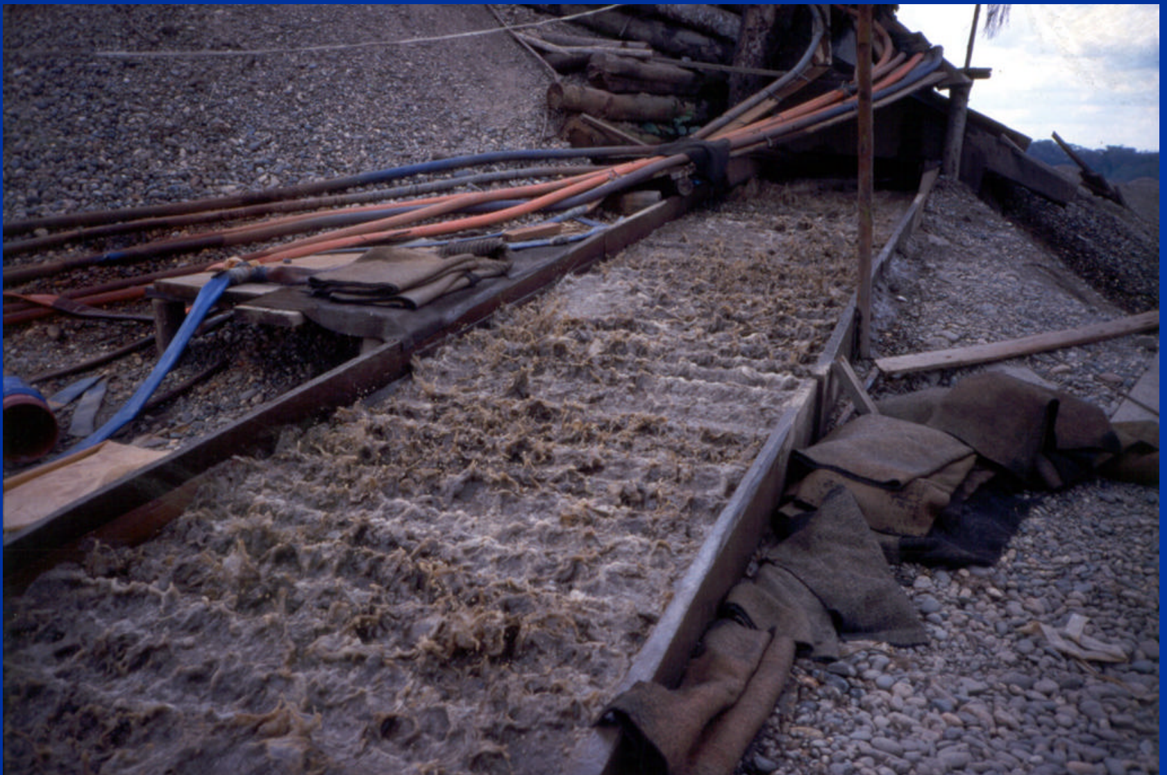
Riffeled sluice box (for coarse gold)
