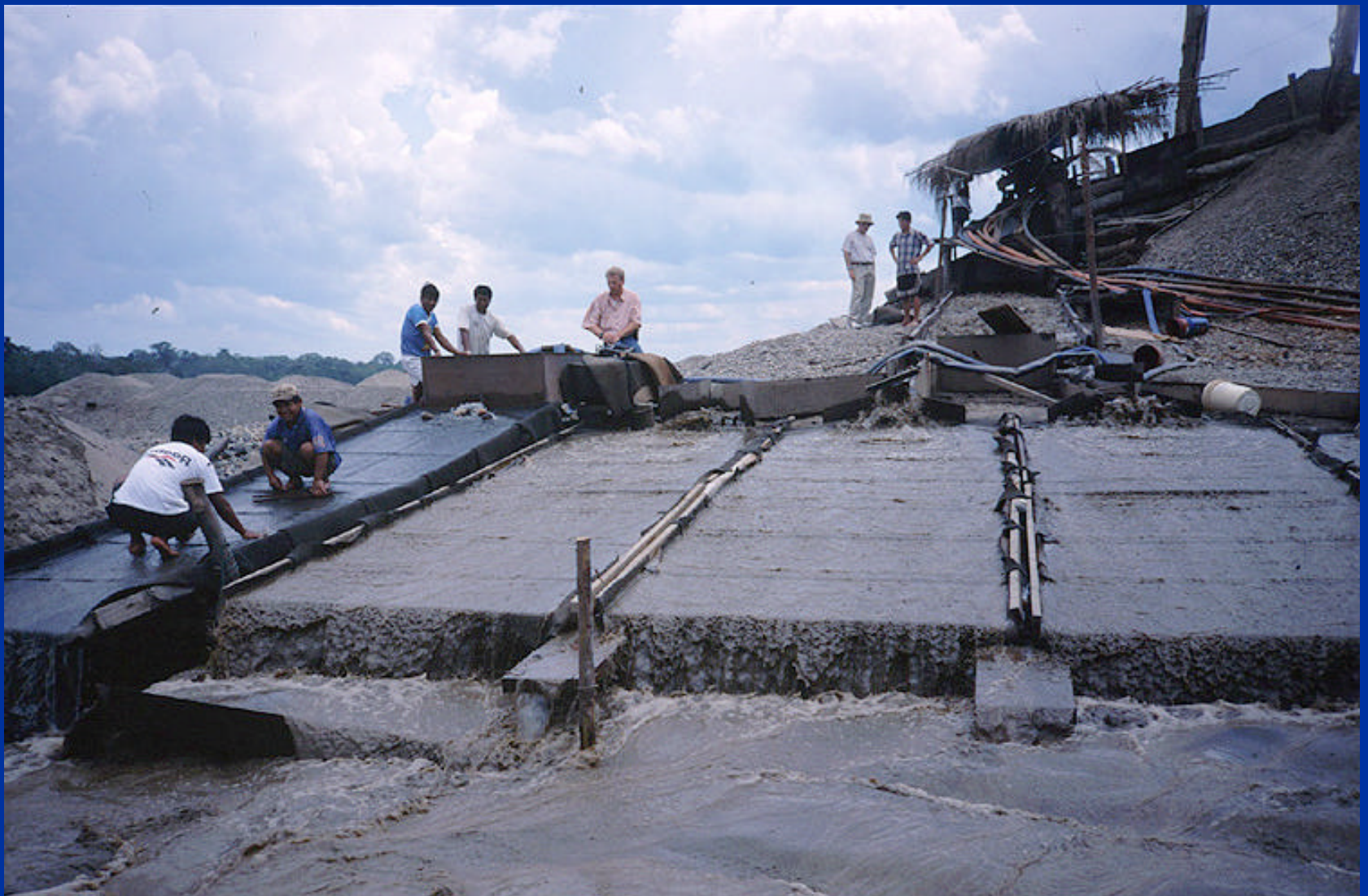
„carpet-only“ sluicebox for fine alluvial gold (see re-cleaning sluice left)
