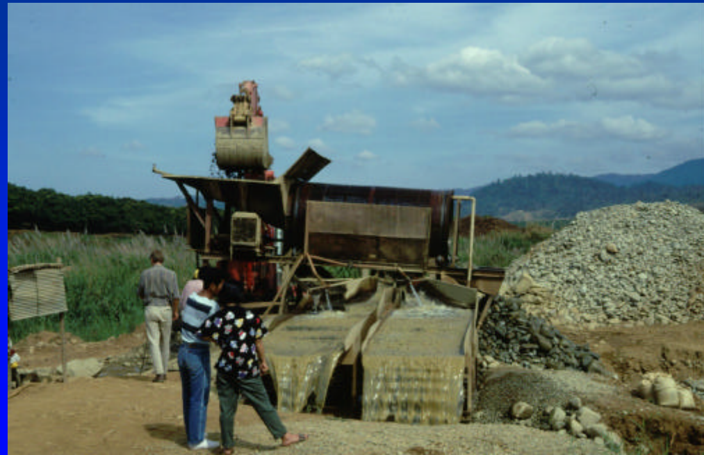
Jig (Ruby mining), combined with scrubber/trommel screen
