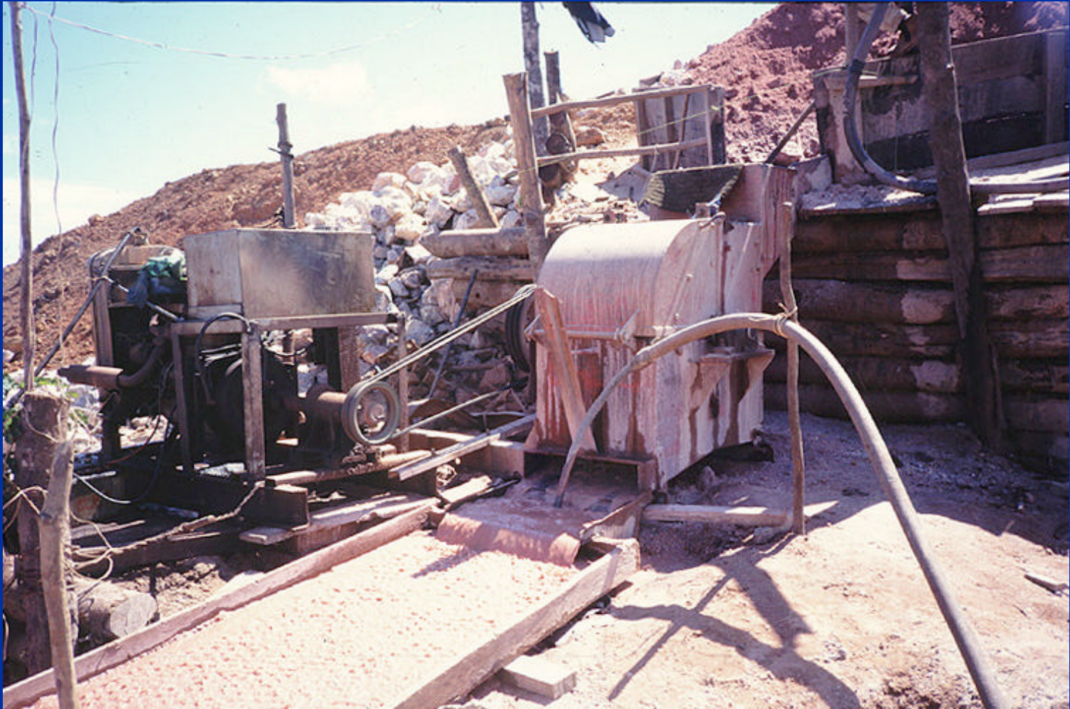
Large hammer mill (2,5t/h)
