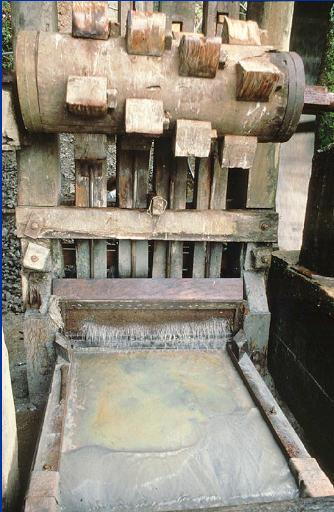
Stamp mill (wooden, driven by water wheel)
