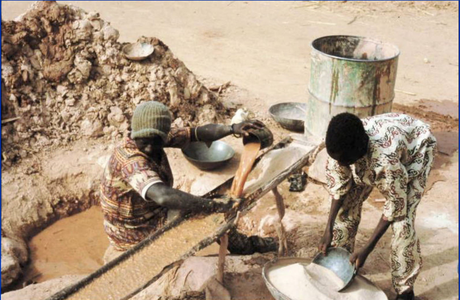
Sluice box (manual)
