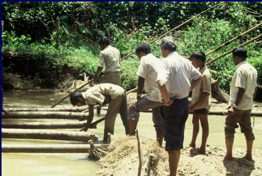
Gems are also mined from riverbed material by a method of dredging with mammoties having long handles.
