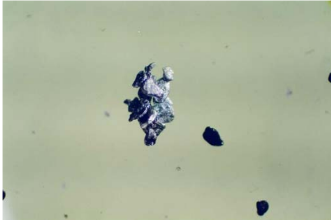
Gold amalgam cluster recovered from sluice box tailings in Suriname. Nominal magnification 40X.
