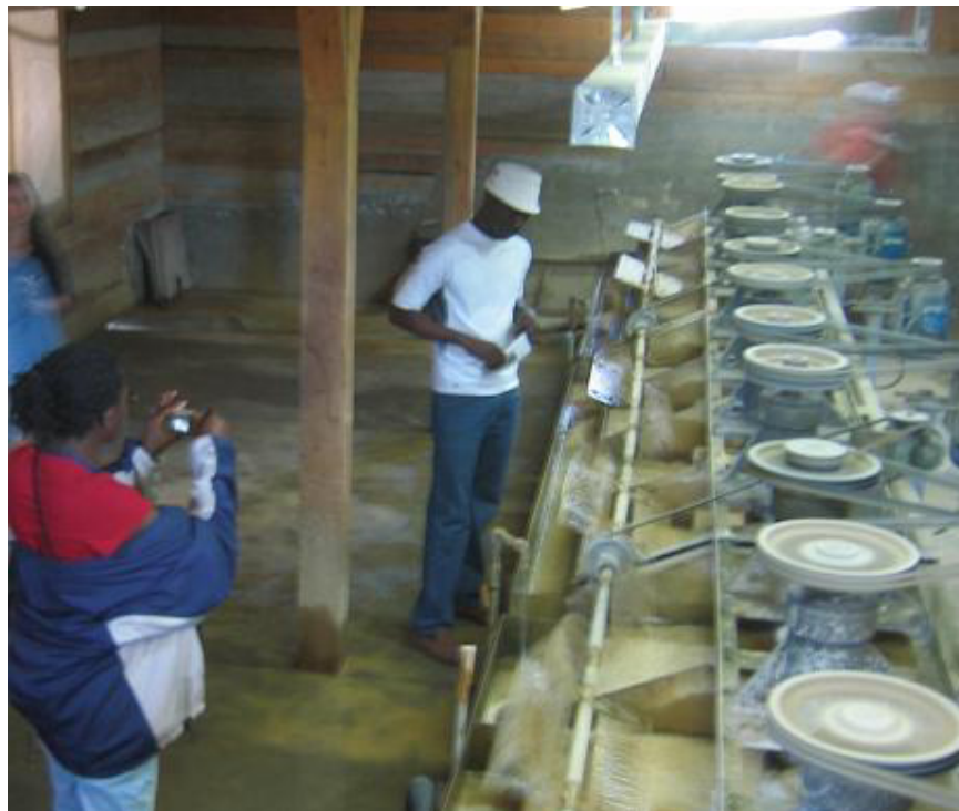
Inspecting the flotation system
