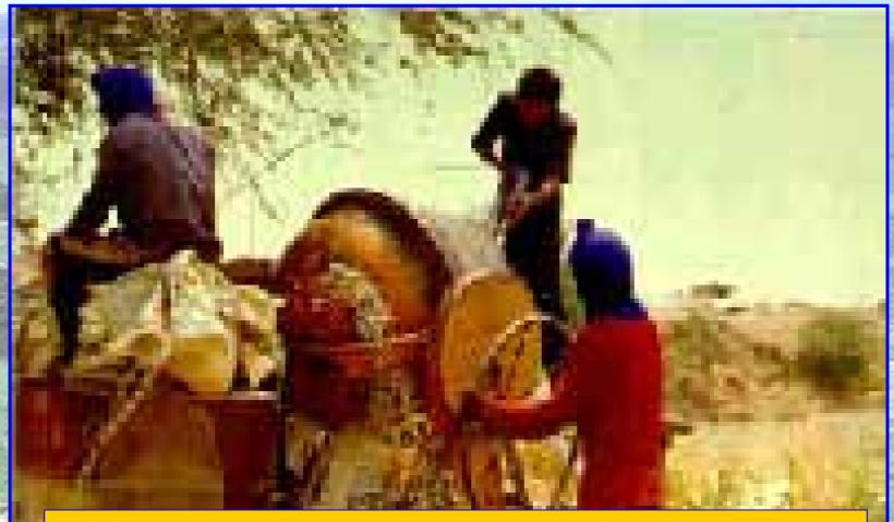
Using the hose duct of 2 inches to transmit high pressure water to the nozzle of ½ inches to wash the sediments in the trommel while revolving.
