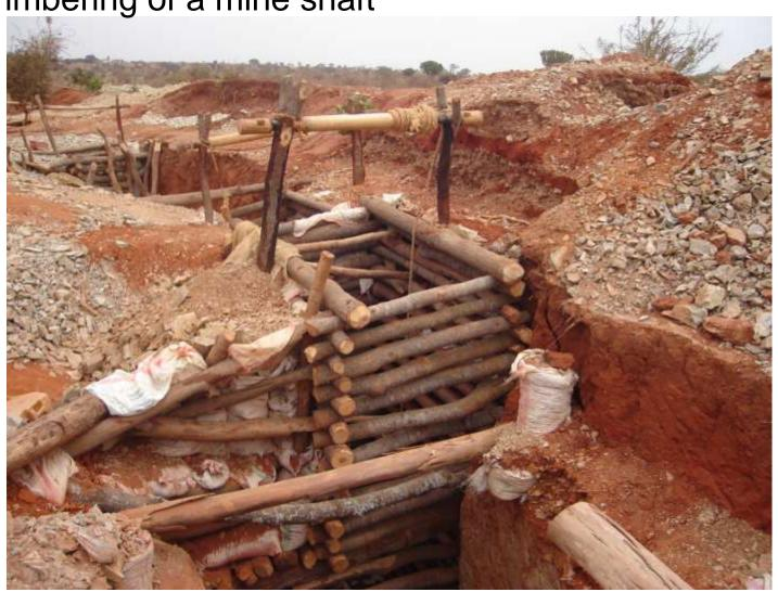
Manual winding shaft for haulage of ore from pits
