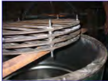
Strips of flat bar steel (40 mm width and 10 mm spacing) are welded to a flat ring.
