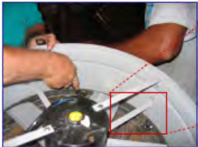
Strips of flat bar steel (40 mm width and 10 mm spacing) are welded to a flat ring.
