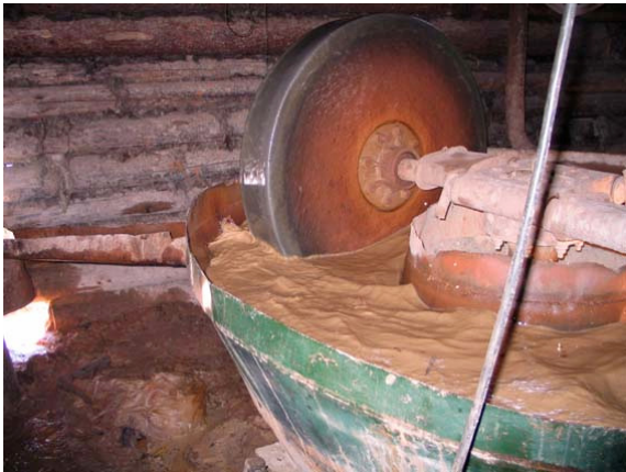
Fig. 1. Milling of hard rock gold ore. About one kilo of mercury is added per three to four tonnes of ore
