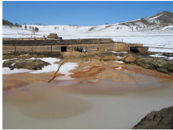
Fig. 2. Tailing from milling of hard rock gold ore
