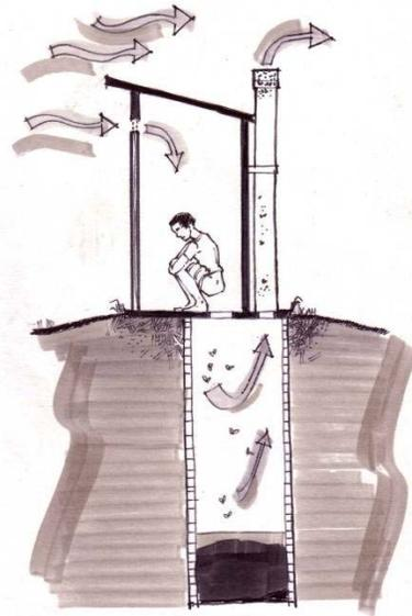
Fig. 10.5 - Ventilated pit latrines (VIP) are host to only 1% of the flies that are attracted to simple pit latrines.
