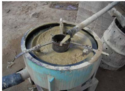
Fig. 4.12 – ABJ centrifuge operating in Zimbabwe
