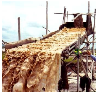
Fig. 4.2 - Monitor pump fed sluice in Indonesia. Note the turbulent flow which limits recovery of fine gold
