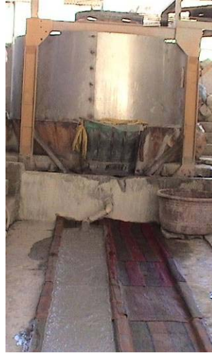
Fig. 4.6 – Ground ore from a Chilean pan feeding alternating sluice boxes with carpet (Ecuador)
