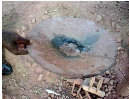
Fig. 4.19 - Riveted shallow batea made of sheet metal (Brazil).
