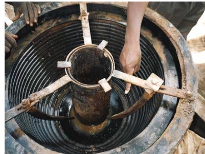
Fig. 4.13 – Rubber cone with ribs (ABJ centrifuge)
