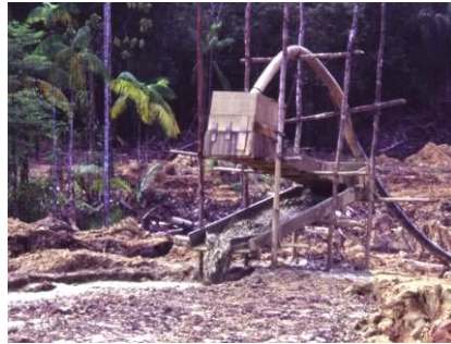
Fig. 4.7 - Pump-fed zigzag sluice in Suriname
