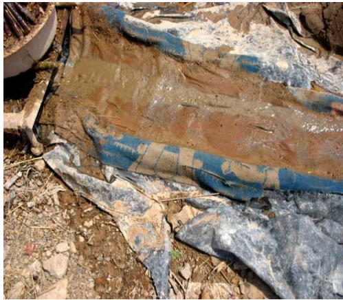
Fig. 4.5 - Clogged trapping mechanism (blanket) of hand-fed sluice
