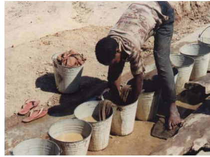
Fig. 4.8 - Cleaning up Hessian carpets using a series of buckets
