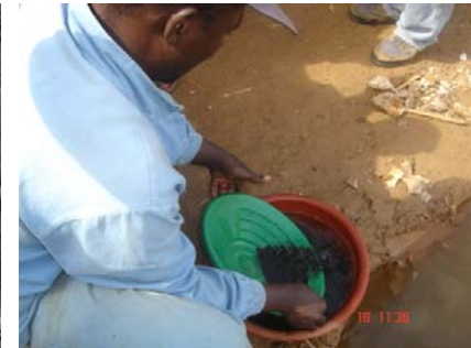
Fig. 4.20 - North American plastic pan with riffles in the side (Mozambique).
