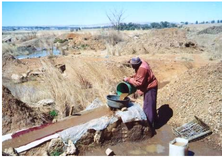
Fig. 4.1 - Hand fed sluice in South Africa
