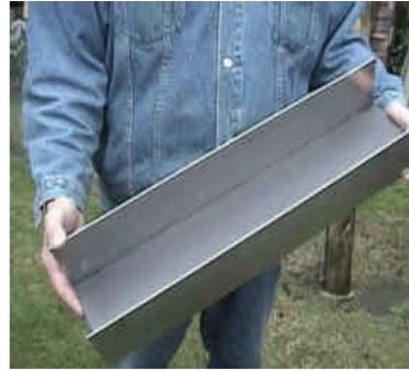
Fig. 4.10 – Cleangold magnetic sluice
