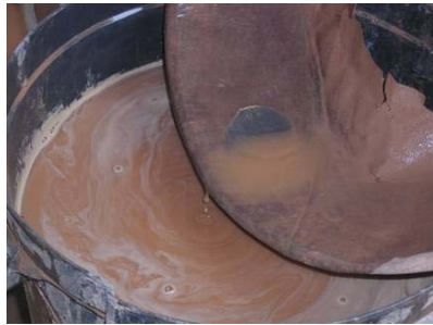
Fig. 4.15 - Miners can capture fine gold even in a very worn out pans (Tanzania).
