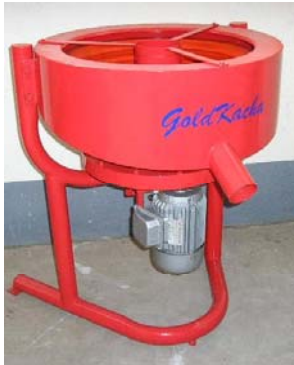
Fig. 4.14 -- Small Mining Supplies (Harare) new centrifuge, the "GoldKacha"
