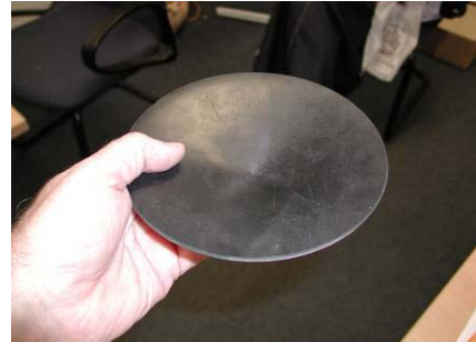
Fig. 4.22 - Small rubber coated cone-shaped batea for testing ore (Peru).
