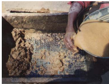
Fig. 4.4 - Feed box for hand fed sluice: mixing ore with water
