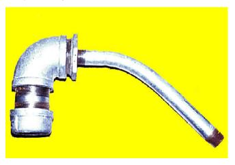
Retorts can reduce drastically mercury emissions Home-made retorts are not expensive. They can be made with water pipes and connections (devised by R. Hypolito)
