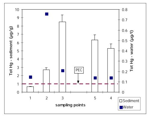
**Figure 3 - Total mercury in Rora and Apopre rivers sediments & waters** (sampling points, up- to downstream: 1 - 3: Apopre; 5 - 4: Rora)
