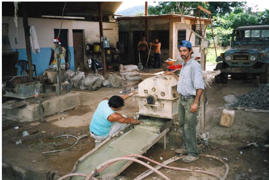
Fig. 2 - Hammer mill and copper-amalgamating plates
