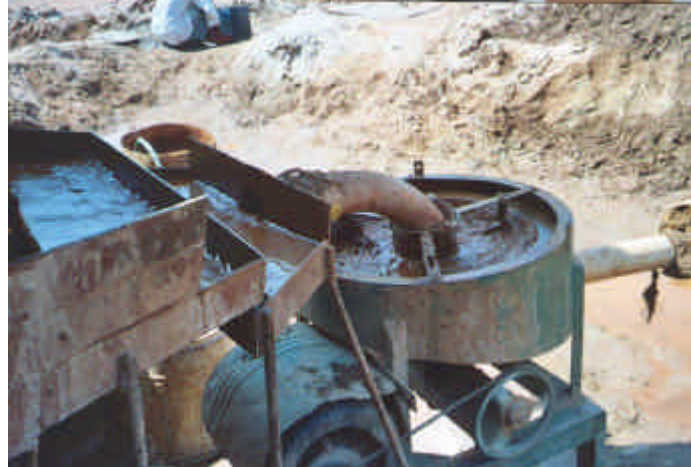
Fig. 7 – Zimbabwean Centrifuge to Concentrate Gold
