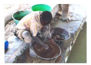
Fig. 3 – Amalgamation of gravity concentrates in Rwamagasa
