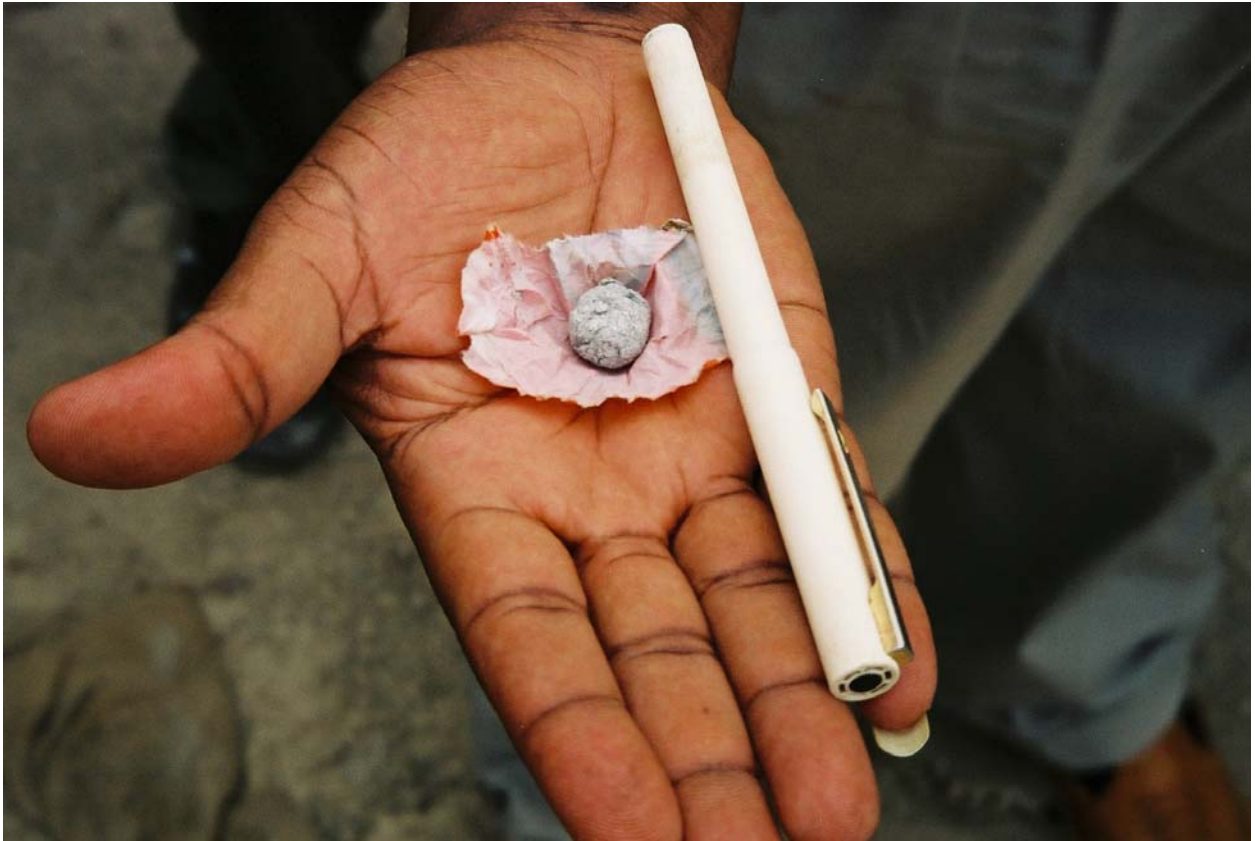
Plate 12. Amalgam placed in paper for burning in charcoal fire (Blue reef mine).
