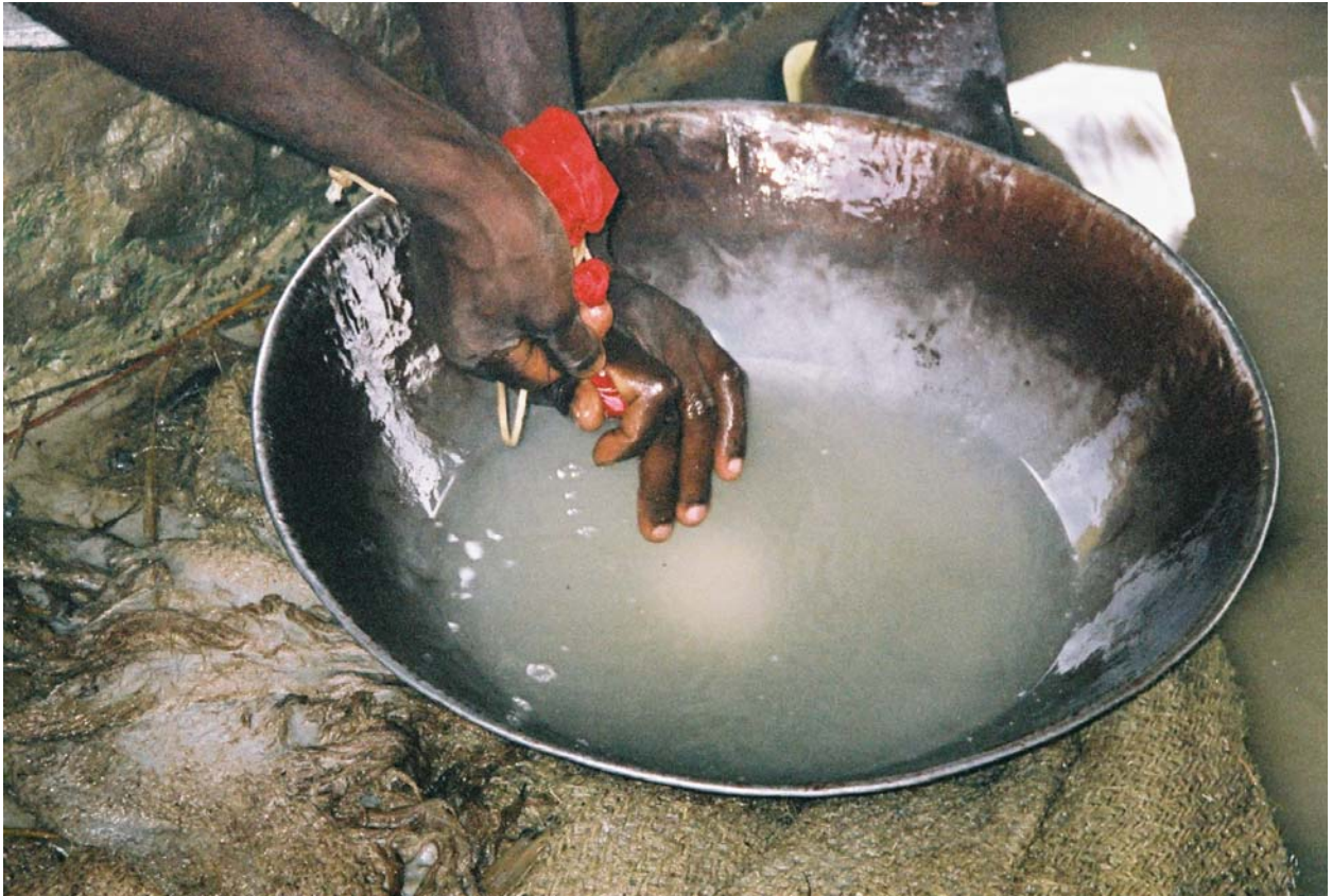
Plate 11. Squeezing cloth to remove excess mercury (Blue Reef Mine)
