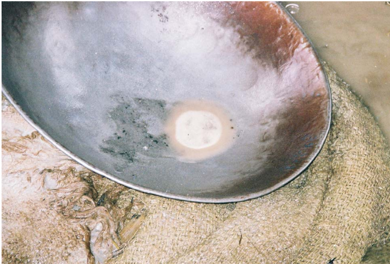
Plate 9. Residual mercury and amalgam at end of amalgamation process (Blue Reef Mine)
