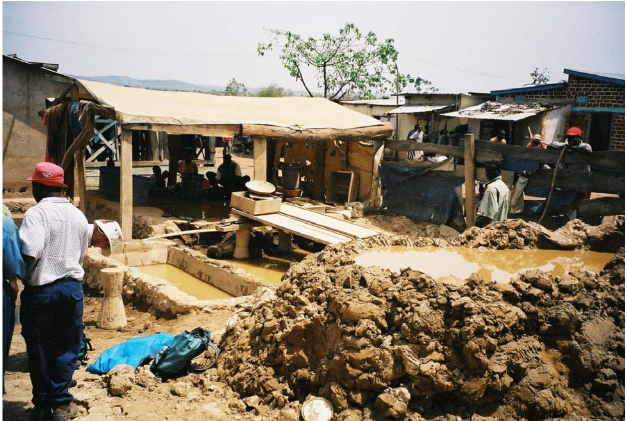
Plate 31. Sluicing and covered amalgamation pond located within the built-up part of Rwamagasa (site A9)
