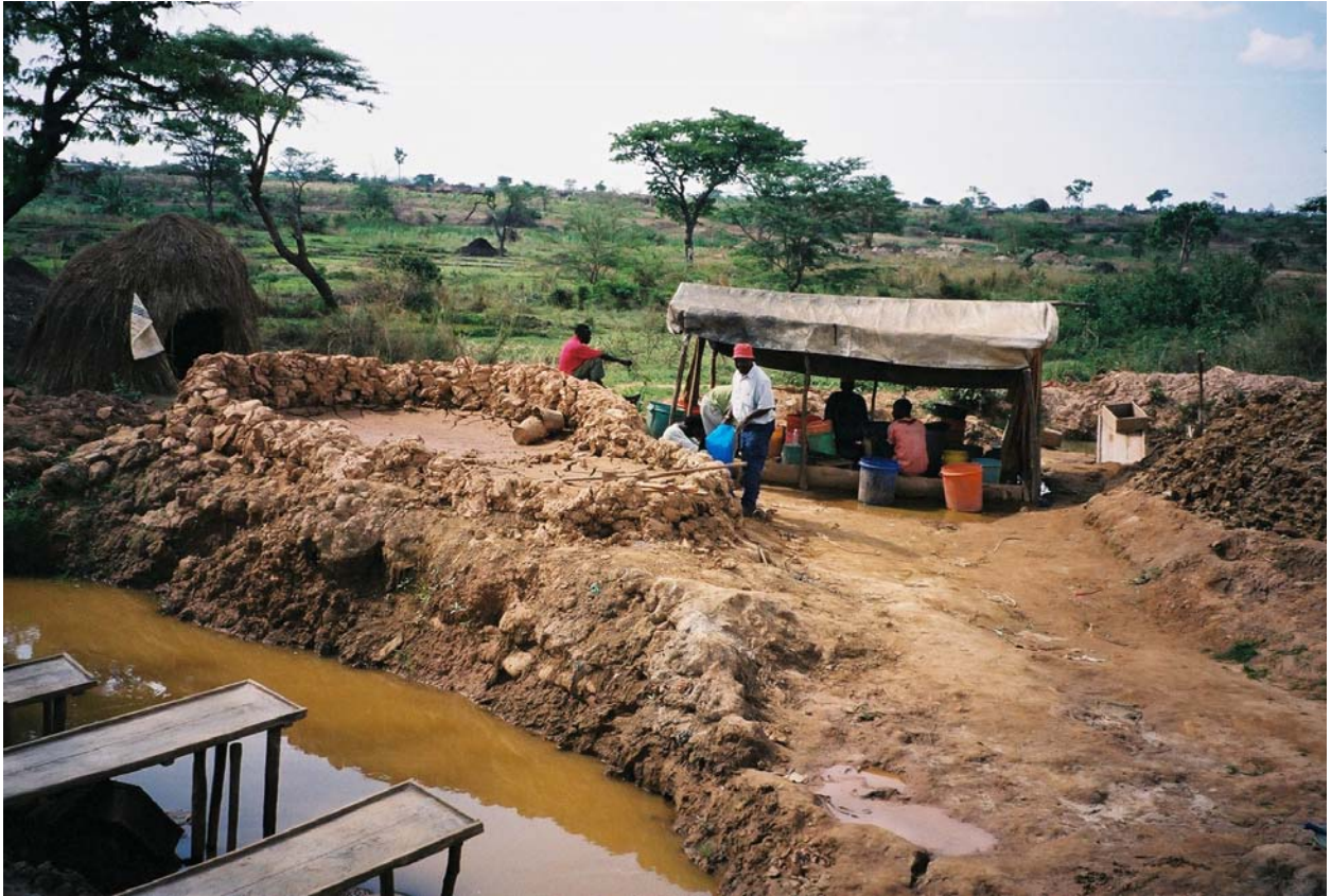
Plate 15. Covered amalgamation pond and sluices at tailings reprocessing site (A031) overlooking the mbuga of the River Isingile.
