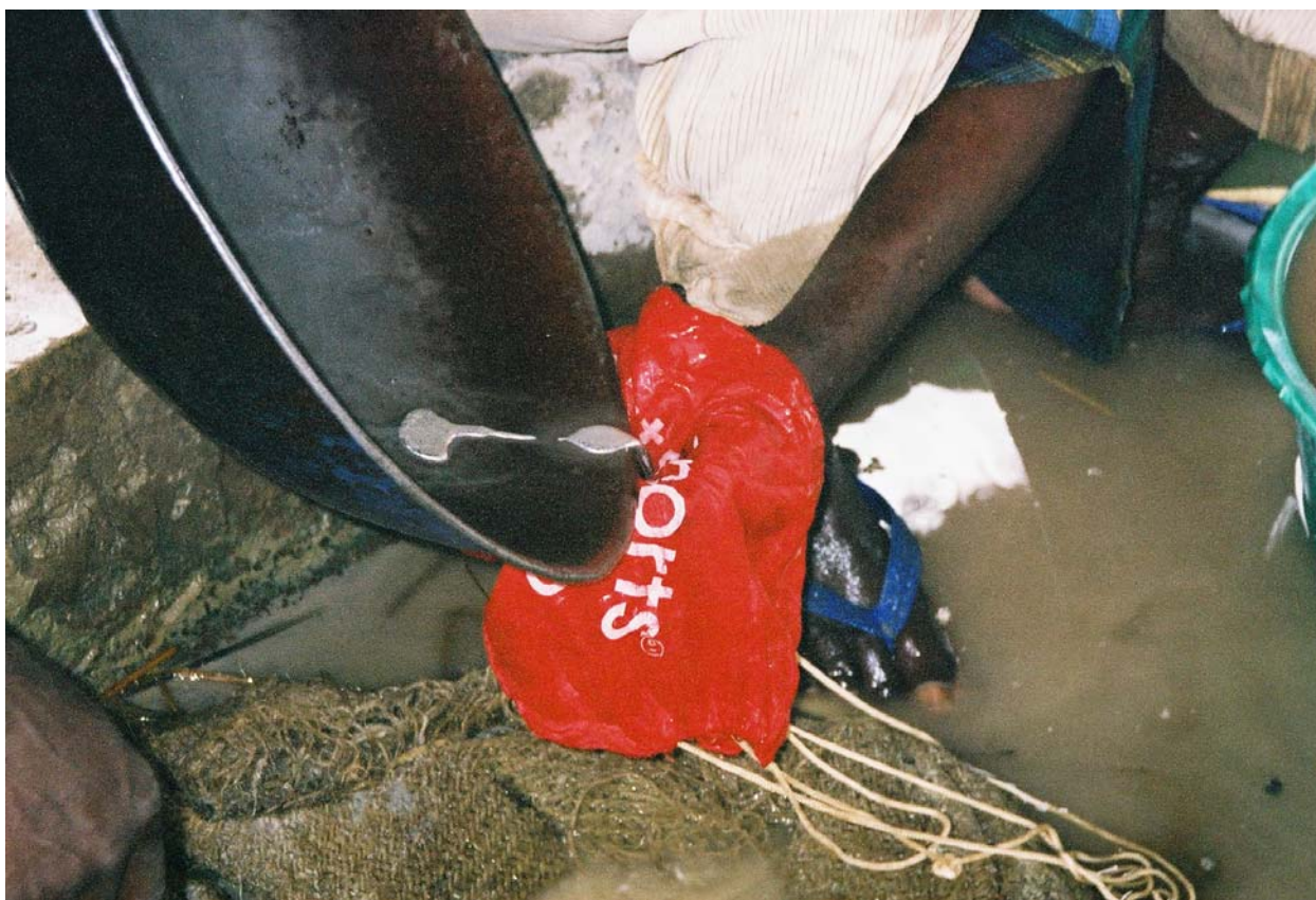
Plate 10. Decanting mercury and amalgam into cloth for removal of excess mercury by squeezing (Blue Reef Mine)
