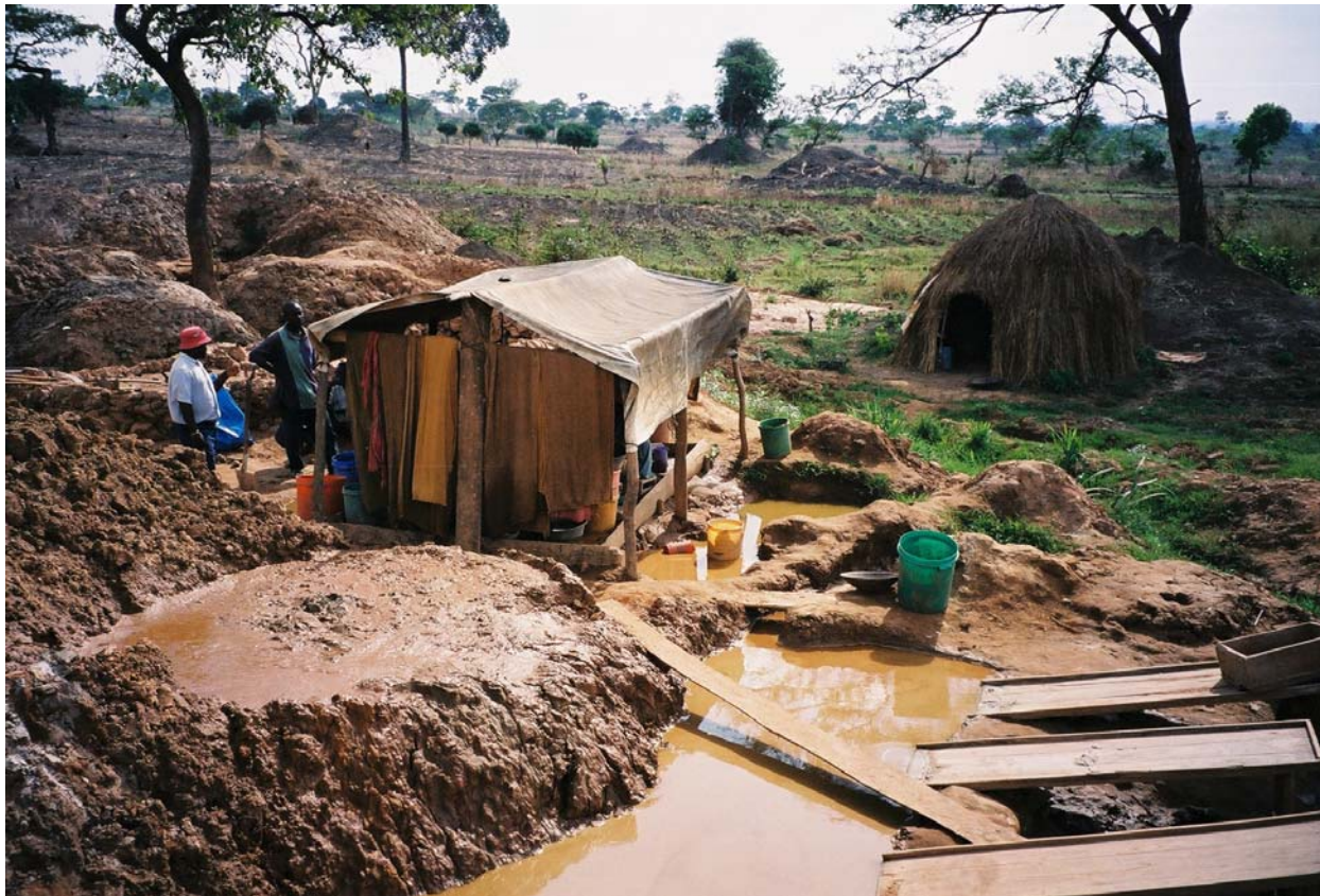
Plate 17. Covered amalgamation pond and sluices at tailings reprocessing site (A031) overlooking the mbuga of the River Isingile.
