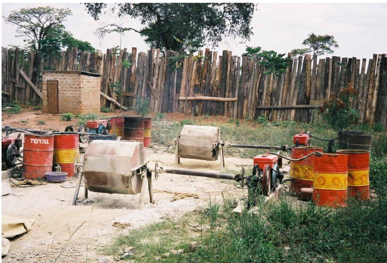
Plate 6. Petrol motor-driven ball mills in fenced mineral processing compound, Blue Reef mine, Rwamagasa
