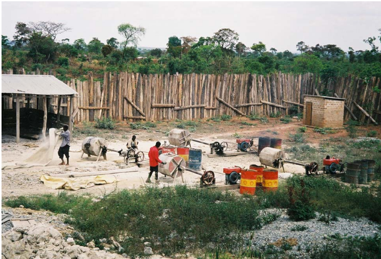
Plate 5. Ball mills in fenced mineral processing compound, Blue Reef mine, Rwamagasa
