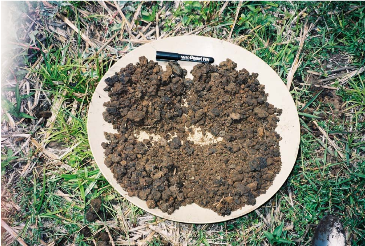
Plate 40. Homogenised and quartered soil sample after disaggregation and mixing (see Plate 46 above)
