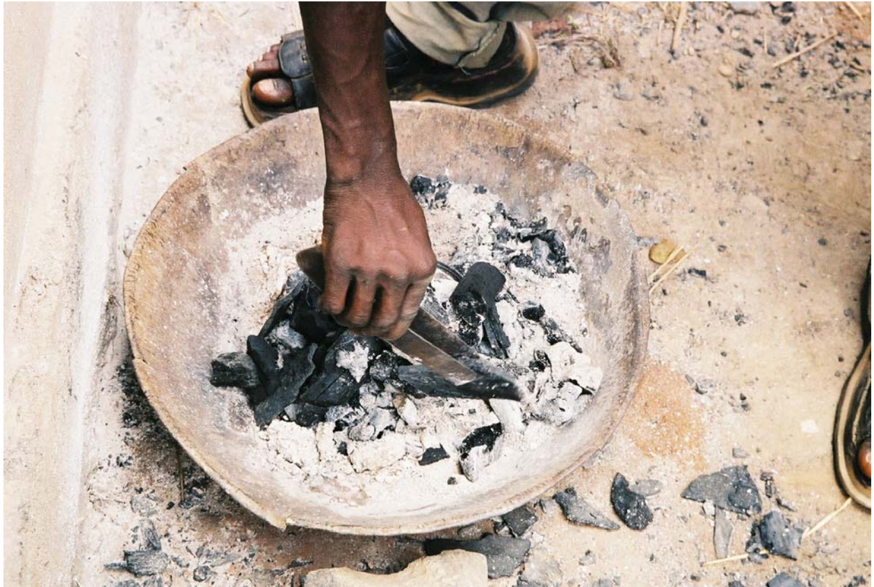
Plate 13. Burning amalgam in charcoal fire to drive off mercury (Blue Reef mine)
