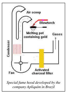
In 1989, a Brazilian company, Apliquim, developed a mercury condensing fume-hood consisting of a series of condensing plates coupled with iodide impregnated activated charcoal filters. This equipment reduces mercury emissions by more than 99.9%. Less than 1  $\mu$ g/m<sup>3</sup> (WHO limit for public exposure) of mercury was detected in the exhausting gases of this fume hood.
