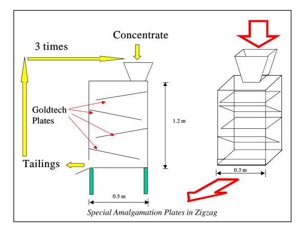
Table 3.10 – Technical Data of a Box with Special Amalgamation Plates in Zigzag
