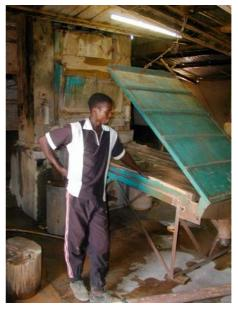
A: Bowl-concentrator B: Copper-plate Illustration 29 - Bowl-concentrator and copper-plate in a closed building at Lilly mill.
