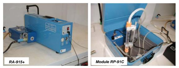
Illustration 13 - The LUMEX RA-915<sup>+</sup> analyser equipped with the RP 91C attachment.
