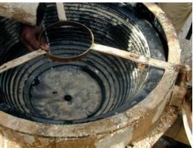
b) Remaining amalgam droplets in the riffles
