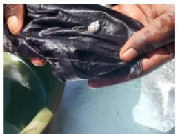
F: Amalgam after squeezing to remove unused mercury
