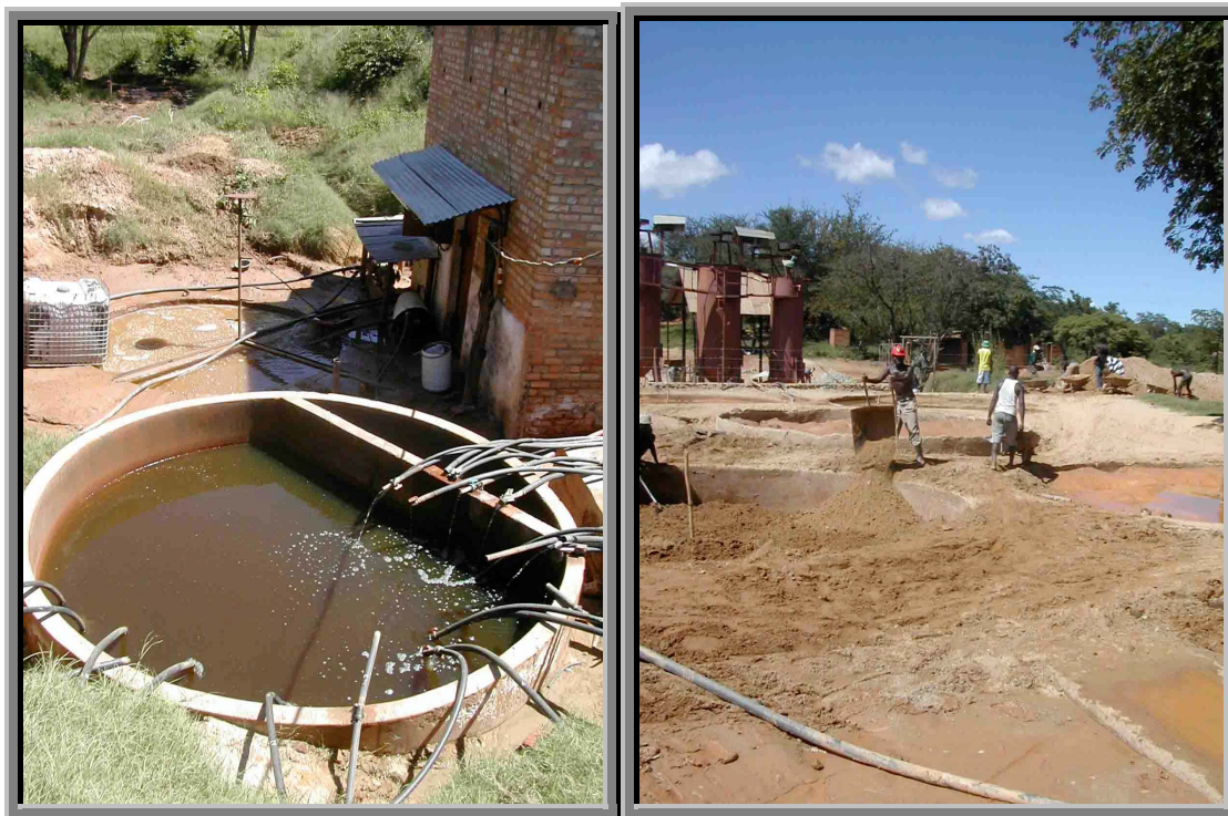
Picture 8 - Amber Rose mill - tailings; cyanidation tank; pregnant solution; filling the tanks with tailings (end).
