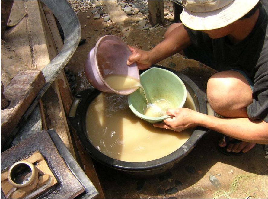
Figure 7 - Recovery of Hg-Au amalgam by rough “panning”
