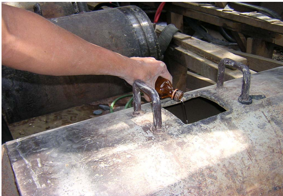
Figure 5 - Pouring mercury into the ball mill
