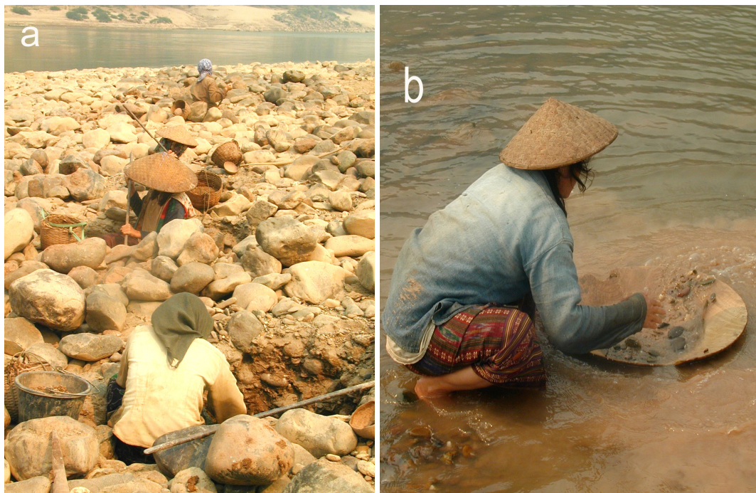
Illustration 6 - (a) Digging of the alluvium in the riverbed of the Mekong (close to Houay Gno); (b) panning of the alluviums.
