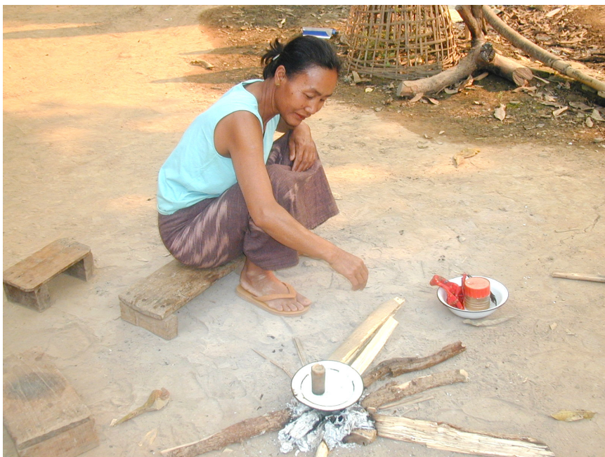
Illustration 9 - Recovery of evaporated mercury in a bamboo tube. The amalgam is covered by the bamboo tube, mercury condense along the walls of the bamboo tube (Pak Ou).
