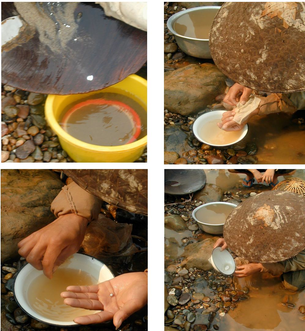
Illustration 7 - (a) Mercury added directly in the pan ( Houay Koh); (b) remove of excess of mercury in a small cloth ( Houay Gno); (c) the amalgam after squeezing; (d) recovery of the excess of mercury.
