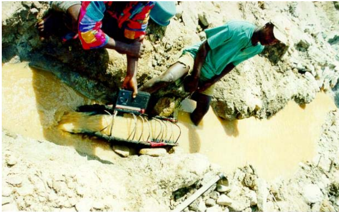
Sluice box built from tree barks in Sussundenga, Manica Province
