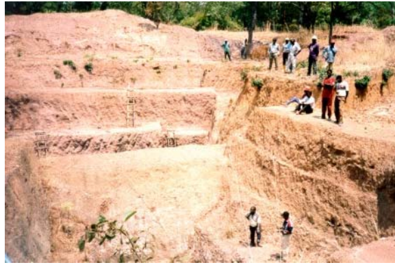
A pit well benched with simple tools in Ndola rural
