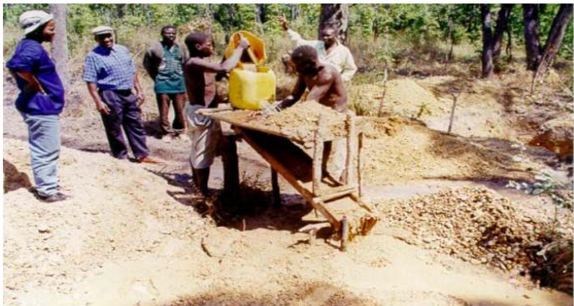
A locally built sluice box, equipped with a 20-litres gallon for water-feed used to recover the gold in N'tulo, Niassa Province
