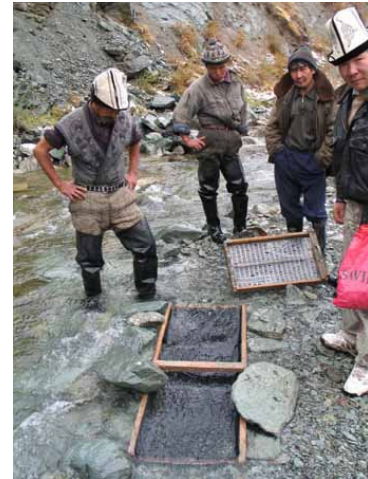
Figure 5. Sieve and sluice
