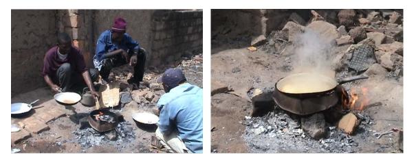
Gold particles are leached with nitric acid to remove iron oxide crusts
