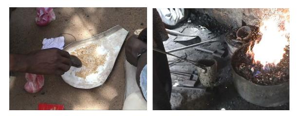
Gold "cleaned" with nitric acid is melted with borax
