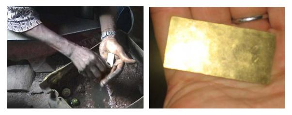
Melted gold is transformed into bars and "cleaned" with lime
